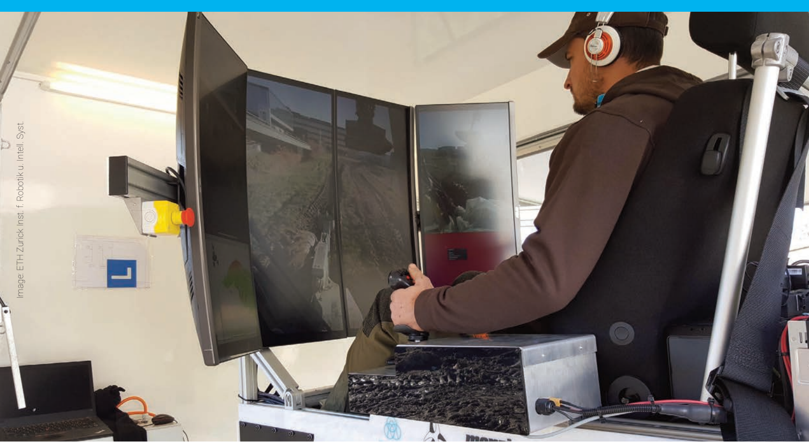
Image 1 | At the Menzi Muck remote-controlled walking excavator the Fastvideo SDK solution allowed up to 60fps of synchronized image acquisition from each of the two 3.1MP cameras.
